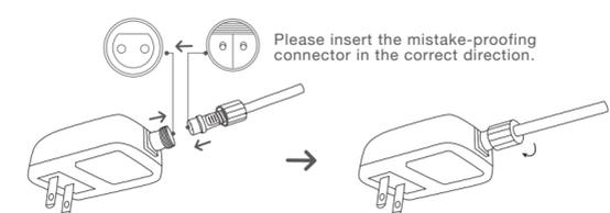
Please insert the mistake-proofing connector in the correct direction.
