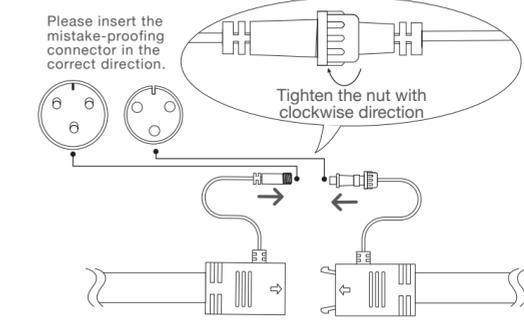
Tighten the nut with clockwise direction
