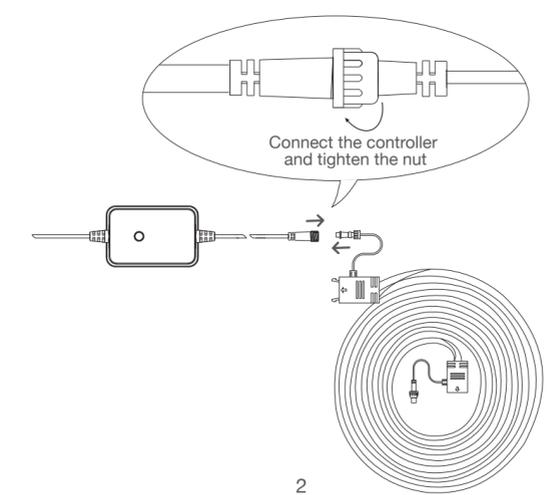
Connect the controller and tighten the nut
